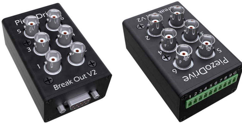
Figure 4. Front and rear views of the breakout box
